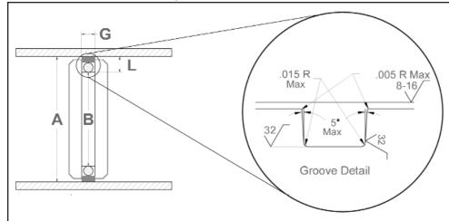
NOTE: Most solid PTFE seals require stretching in order to be installed properly and without damage. Instructions for installation tools are available from the MPI Engineering D e p a r t m e n t .
